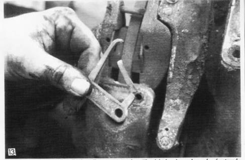
Undo and remove the handbrake caliper retractor plate. The right-hand arm shown has fractured through fatigue. Both will be replaced as a matter of course.
