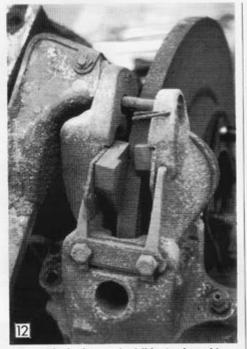
Now the brake area is visible. See how this handbrake pad has slipped from its mount.
