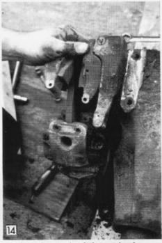
Release the two pivot bolts securing the handbrake caliper and remove.
