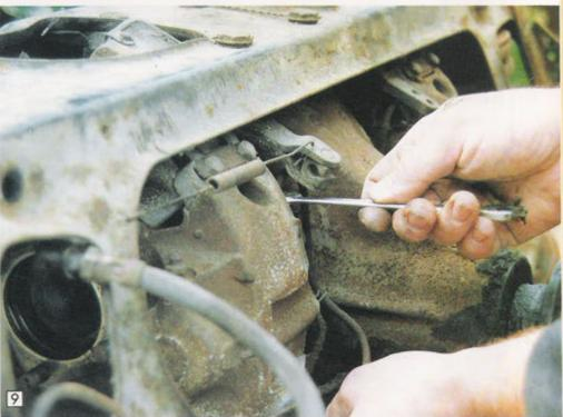
Remove all the brake pipes and the handbrake linkage spring.
