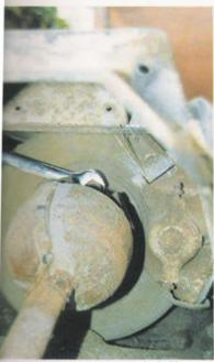
move the four nuts securing the half afts to the output flanges and lift the half
