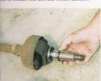
his shows the shim at the outer end of the will shall used to achieve the correct end loat for the hub bearing. These will be focused further during the assembly procedure.
