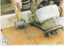
Undo a securing nut to the outer lower fulcrum shaft and tap out the shaft using a drift. The hub carrier can now be lifted
