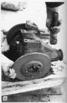
Tap the disc off using a soft-faced hammer.
