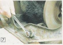
Remove the nuts holding the lower wishbone to the frame and tap out the shaft.
