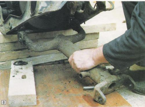
The shaft can now be lifted away. Don't worry about the washers and seals that fall; these will be replaced anyway later on.
