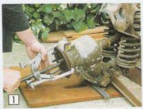
Lock the half shaft in position by inserting a screwdriver or similar through the inner universal joint so that the shaft can't spin. Remove the split pin from the shaft end nut and remove the nut. Using a three-eared puller (or the Jaguar type), free the shaft
