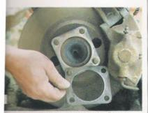
is shows the shims between the flanges sed to obtain the correct wheel camber.
