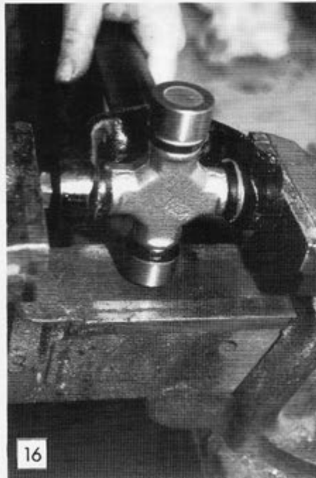
16 Place the universal joint in position and slide into the fitted cup. Place another cup into the vacant hole. Push the two cups home using a vice. You will need to use a spacer (small socket or even a nut will do) to push the cups past the circlip groove. Check that the joint moves freely and then fit new circlips. Do not be surprised if a needle roller falls and obstructs the joint. If this happens then the cups have to be extracted, the roller put back in place and the cups pushed home again. Fit the other section of the driveshaft to the universal joint ensuring that all pre-punched numbers correspond.
