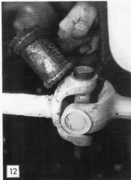
12 Deliver a series of blows with a soft faced hammer to drive the yolk down on the universal joint.
