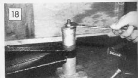
18 Alan has devised a simple tool for installing the bushes. The bottom section shown is the same diameter as the eye in the radius arm. The top is the same diameter as the bush. Through the two runs a threaded rod. The bush is pulled down by the top part of the tool when the thread is tightened. Any machine shop will press the bushes in for you for a matter of a few pounds.
