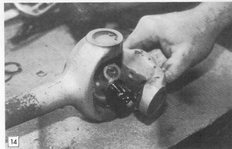
14 Manoeuvre the yolk away from the universal joint and repeat operation 12 for the other half of the universal joint.
