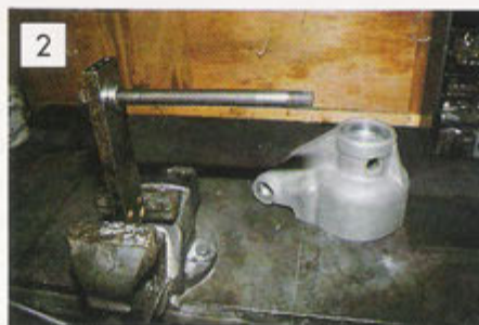
To set up for the assembly procedure it will be necessary to knock-up a simple jig. Use a piece of plate steel approx. 7in x 4in x 3/8in. Drill and tap a hole to receive the lower fulcrum shaft so that the shaft can be retained as shown.
