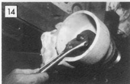
14 Back to our piece of threaded rod. This time it is needed to pull the bearing home.
