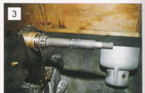
Position a spacer to an approximate size of the lower wishbone outer forks on the shaft first followed by the seating ring for the oil seal, bearing, spacer sleeve and an excess of known size shims and the second spacer sleeve.
