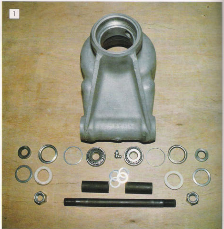
This shows the lower fulcrum shaft with its component parts prior to assembly in the hub carrier. As there is a bearing in each end of the shaft, each side is a mirror of the other. They are fitted on the shaft as follows. Left to right are: the shims to centralise hub carrier in the wishbone, retaining washer on seating ring for the oil seal, container for oil seal and felt seal, seating ring for oil seal, bearing, spacer sleeve and shims fitted between sleeves for pre-load.
