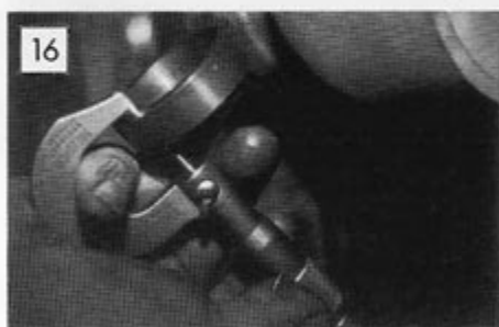
16 Take a piece of machined brass to sit on the bearing centre. Accurately measure its thickness using a micrometer.
