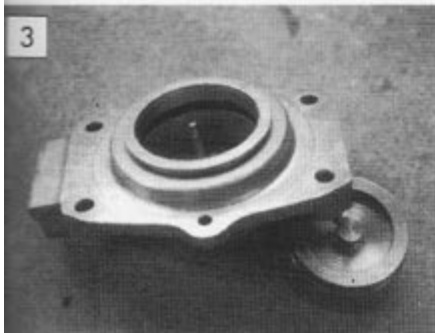
3 With the cylinder thoroughly cleaned the assembly can begin. Coat the inside of the cylinder and the new rubber seal with brake fluid. Ease the seal into its recess in the cylinder wall, making sure that it does not twist and is firmly seated.
