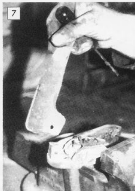
7 To gain access to the handbrake adjuster mechanism, remove the cover by releasing a central screw and a top pin. This will also free the operating lever from the pad carrier.
