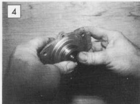
4 Using our new caliper piston (or the old one if it is in a new condition), coat with brake fluid and ease into the bore. Be very careful not to nick the rubber seal. The brake fluid should help it slip into position. It may well be a tight fit as it goes down.
