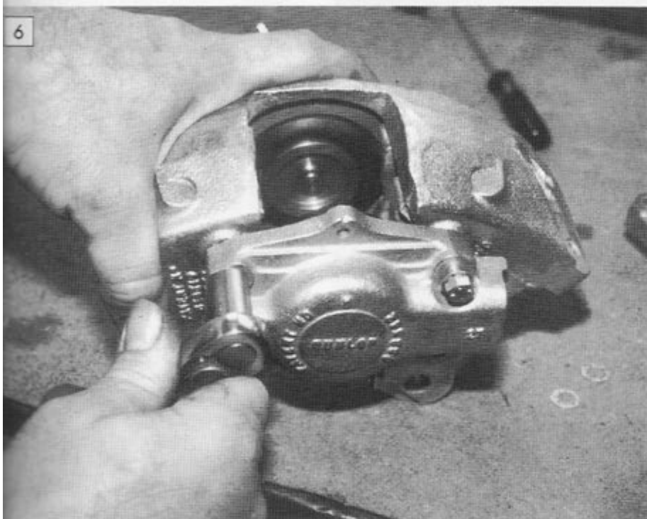
6 Bolt the caliper cylinder on to the main caliper assembly. We used new bolts and washers; the cost is minimal. Use firm and even pressure but don't overdo it - it's a nasty job extracting broken bolts.
