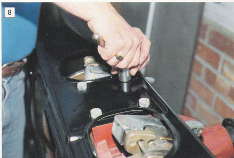
9 Bolt the lower mounting for the inner fulcrum shaft to the differential casing. There are shims used. Here it is a case of putting back what was taken out as the camber adjustment will be made on the drive-shaft. Secure the bolts with locking wire.
