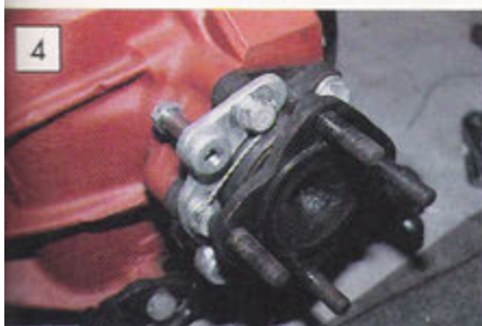
4 The caliper mounting bracket is fitted to the rear of the output shaft.
