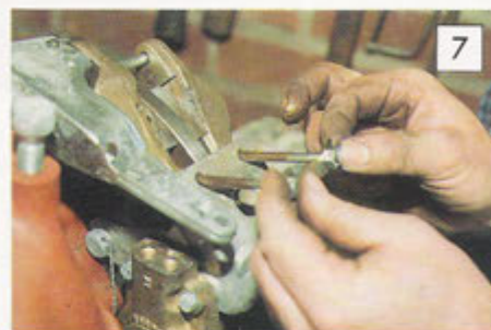
7 Fit the handbrake caliper on to the main caliper and secure with the long pivot bolts and lock tabs. The brass spring yoke goes under the bolt heads with the prongs located in the handbrake calipers.
