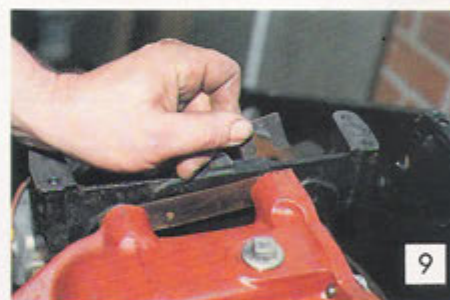
9 Bolt the lower mounting for the inner fulcrum shaft to the differential casing. There are shims used. Here it is a case of putting back what was taken out as the camber adjustment will be made on the drive-shaft. Secure the bolts with locking wire.
