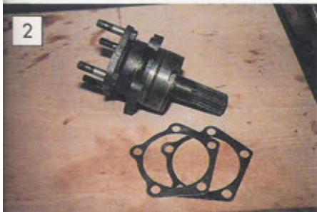
2 New bearings and 'O' ring have already been pushed on to this output shaft.
