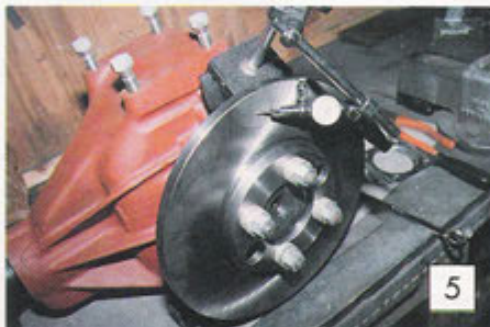
5 Using temporary spacers, fit the disc in place and fully tighten the nuts. If using an old disc, check for run-out with a dial gauge as illustrated.
