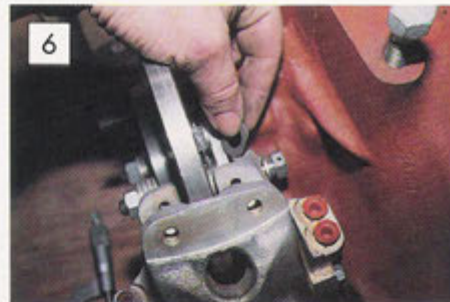
6 The caliper can now be fitted to its carrier and centralised over the disc, using shims to adjust.
