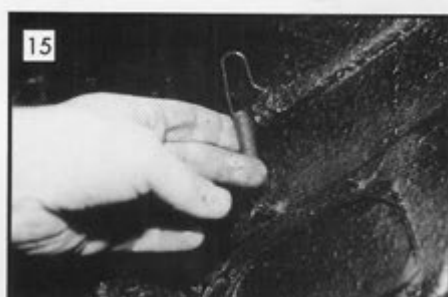
15 Don't forget to replace the spring that supports the handbrake cable. Hook this over the cable only when the rear end is secured.
