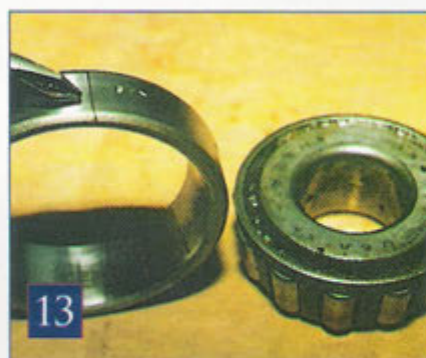
Here's a fault that was unlikely to have been caused by the collision. This outer fulcrum bearing track has cracked. Our work in this area was well timed.
