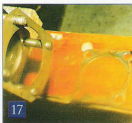
These are the shims used between the output shaft and drive shaft to determine rear camber.
