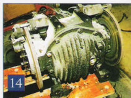
Every item has now been stripped from the cage. The differential unit was the last to be removed seen here with the vacant hole for the electronic speedometer pick up.
