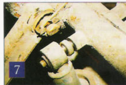
7 Note the spacer washer between the lower wishbone and the shock absorber. The shaft taps through and is completely removable.
