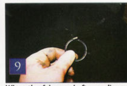
9 When the fulcrum shaft was dismantled, it was found that this grease seal had been split for some time. Grease would soon have vacated the area.
