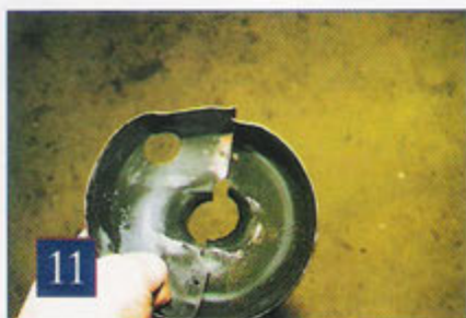
The universal joint cover received some damage but was repairable and would be used again.
