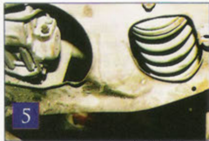
5 See how the frame has buckled in the region between the damper and differential.
