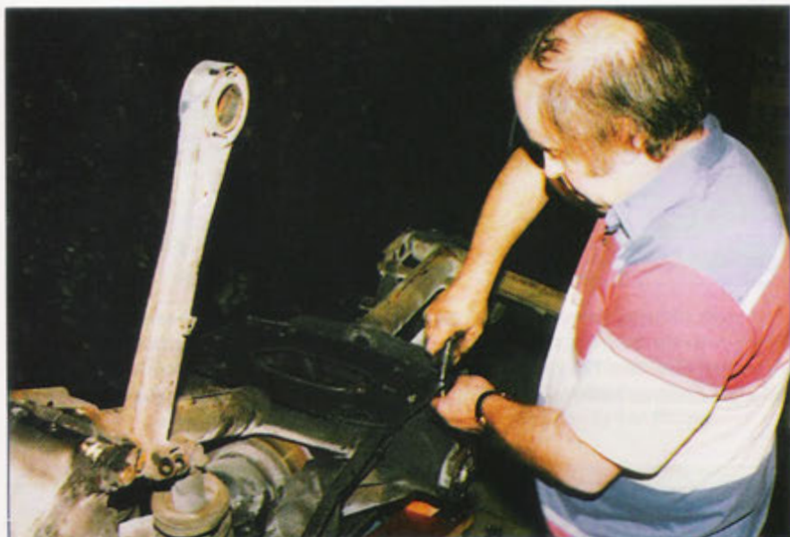
4 Work begins as the bottom pan is undone to give access to the wishbones and diff.
