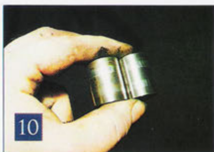
Although showing some slight wear, the inner fulcrum bearing tubes were still in good condition. They were replaced as a precaution, however.
