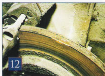
A definite candidate for replacement whether the axle had been stripped or not, these discs are in pretty poor condition.
